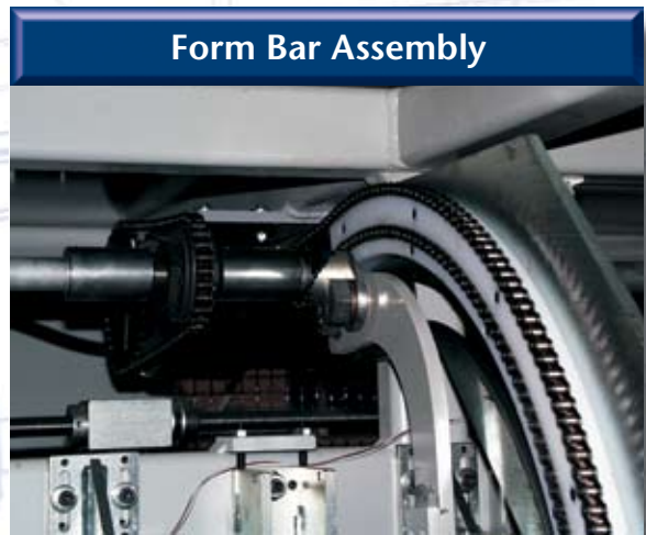
The unique chain-driven, forming bar mechanism ensures concentricity and has electronic variable speed control.
