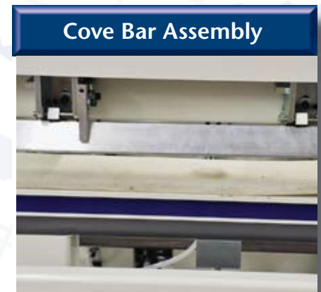
Aluminum cove bar with electronic temperature controls and 90° stops.
