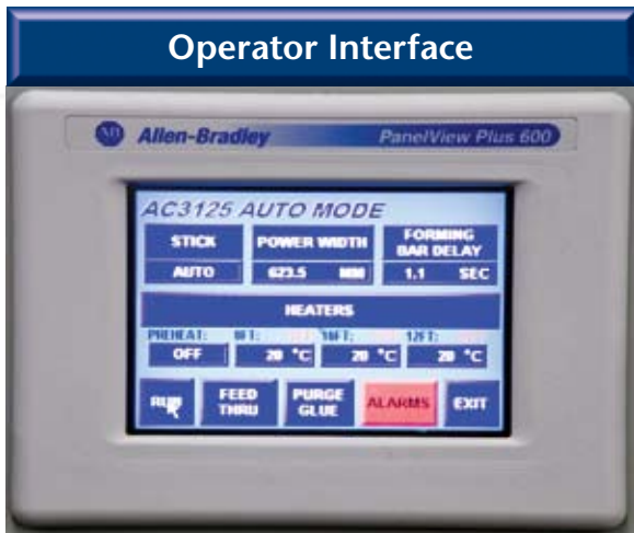
Operator interface with color monitor and PLC controlled sequence of operation.
