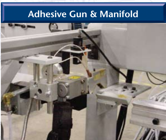
Proprietary 3-bead manifold design with air-actuated adhesive gun.
