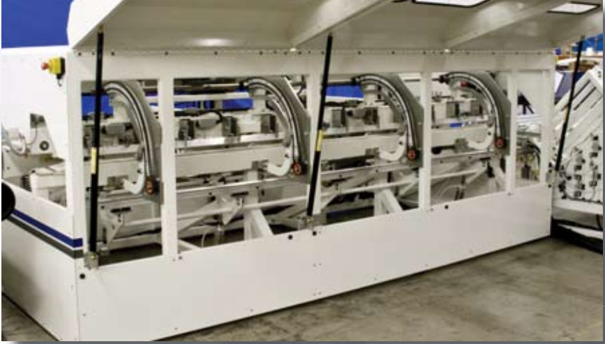
Form bar assembly is electronically driven with chains at four (4) points and includes electronic variable speed control.
