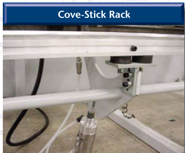
Aluminum cove-stick placement rack with five (5) pneumatic cylinders securely places cove-stick in backslash.
